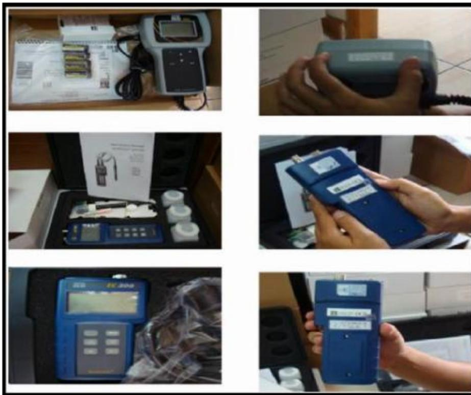
Gambar 46. Contoh Sarana Alat Bantu Penyuluhan (DO Meter, pH Meter, Salinity Meter)
